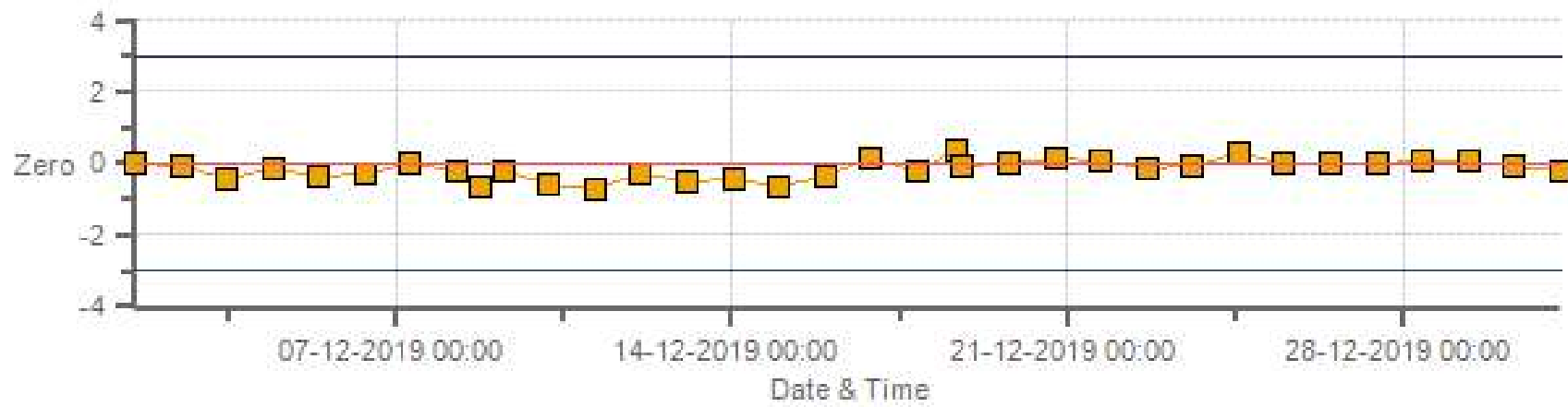
H2S [ppb] Calibration: LICA Maskwa Monthly: 12-2019 Type: Zero
