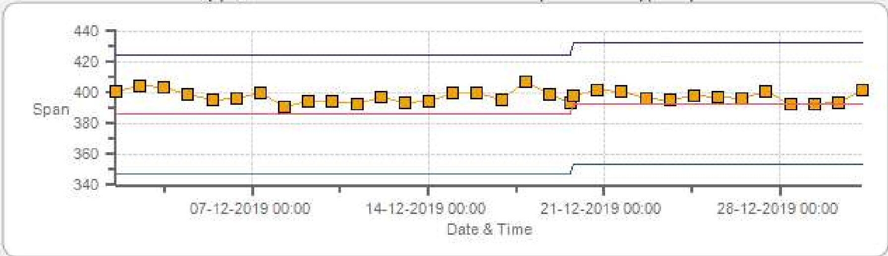
NOx [ppb] Calibration: LICA Maskwa Monthly: 12-2019 Type: Span
