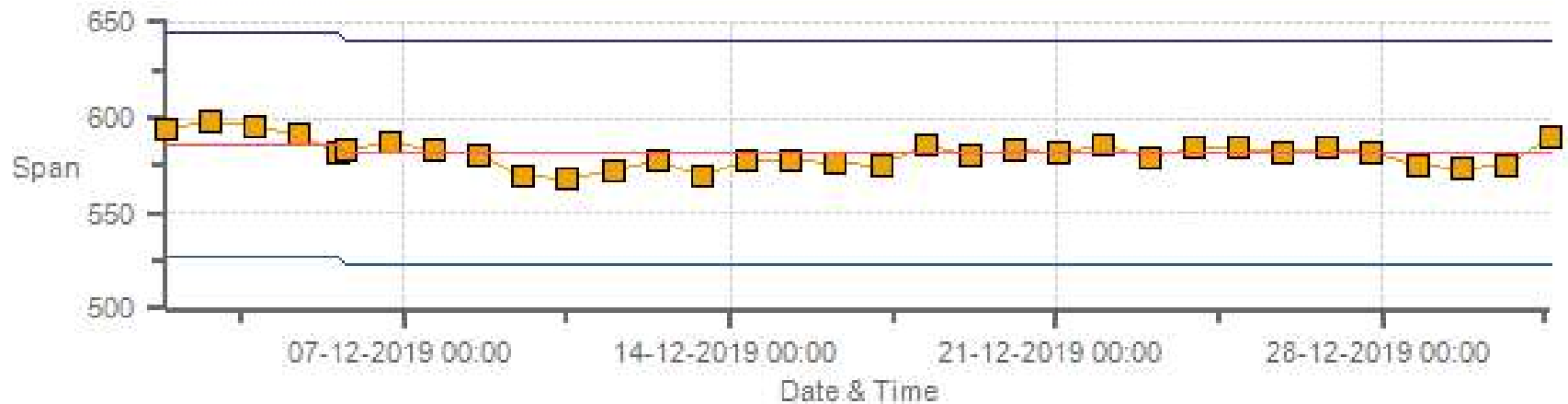
SO2 [ppb] Calibration: LICA Bonnyville-East Monthly: 12-2019 Type: Span
