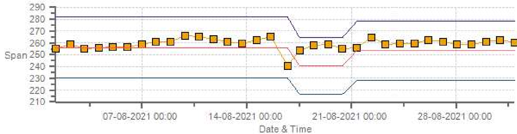
NOX[ppb] Calibration: Cold Lake South Monthly: 08-2021 Type: SpanAndZero - Span
