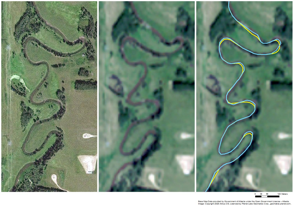
Figure 3. Example of the spatial inaccuracies associated with stream boundaries, where the location of the stream centre line does not match the actual location of the stream and exceeds the 5 m accuracy tolerance in the SPOT imagery. In this example, the yellow lines represent the location of the streamline from the provincial data and the blue line represents the manually edited location of the new stream centre line.
