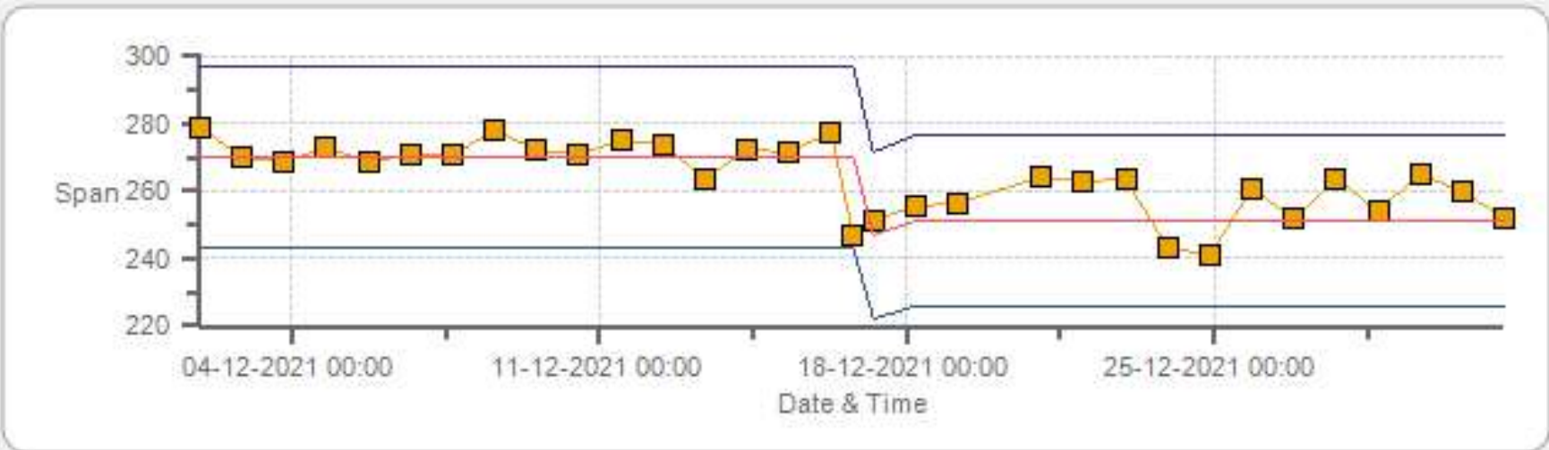
NOX[ppb] Calibration: Cold Lake South Monthly: 12-2021 Type: SpanAndZero - Span
