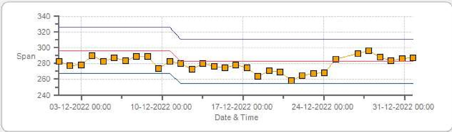
NO2[ppb] Calibration: Cold Lake South Monthly: 12-2022 Type: SpanAndZero - Span
