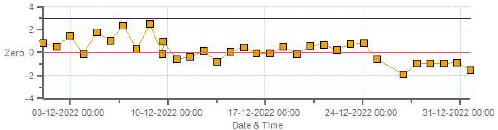
O3[ppb] Calibration: Cold Lake South Monthly: 12-2022 Type: SpanAndZero - Zero
