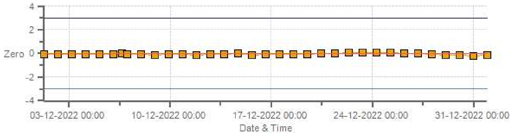
SO2[ppb] Calibration: Lac La Biche Monthly: 12-2022 Type: SpanAndZero - Zero
