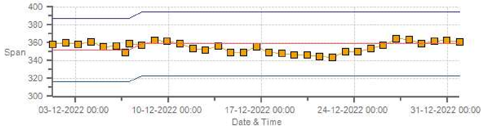
NOX[ppb] Calibration: Lac La Biche Monthly: 12-2022 Type: SpanAndZero - Span
