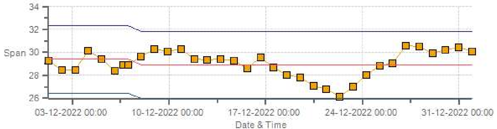
H2S[ppb] Calibration: Lac La Biche Monthly: 12-2022 Type: SpanAndZero - Span
