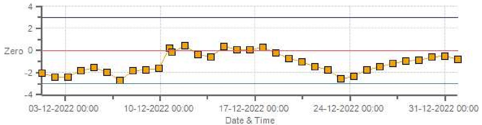
H2S[ppb] Calibration: St. Lina Monthly: 12-2022 Type: SpanAndZero - Zero
