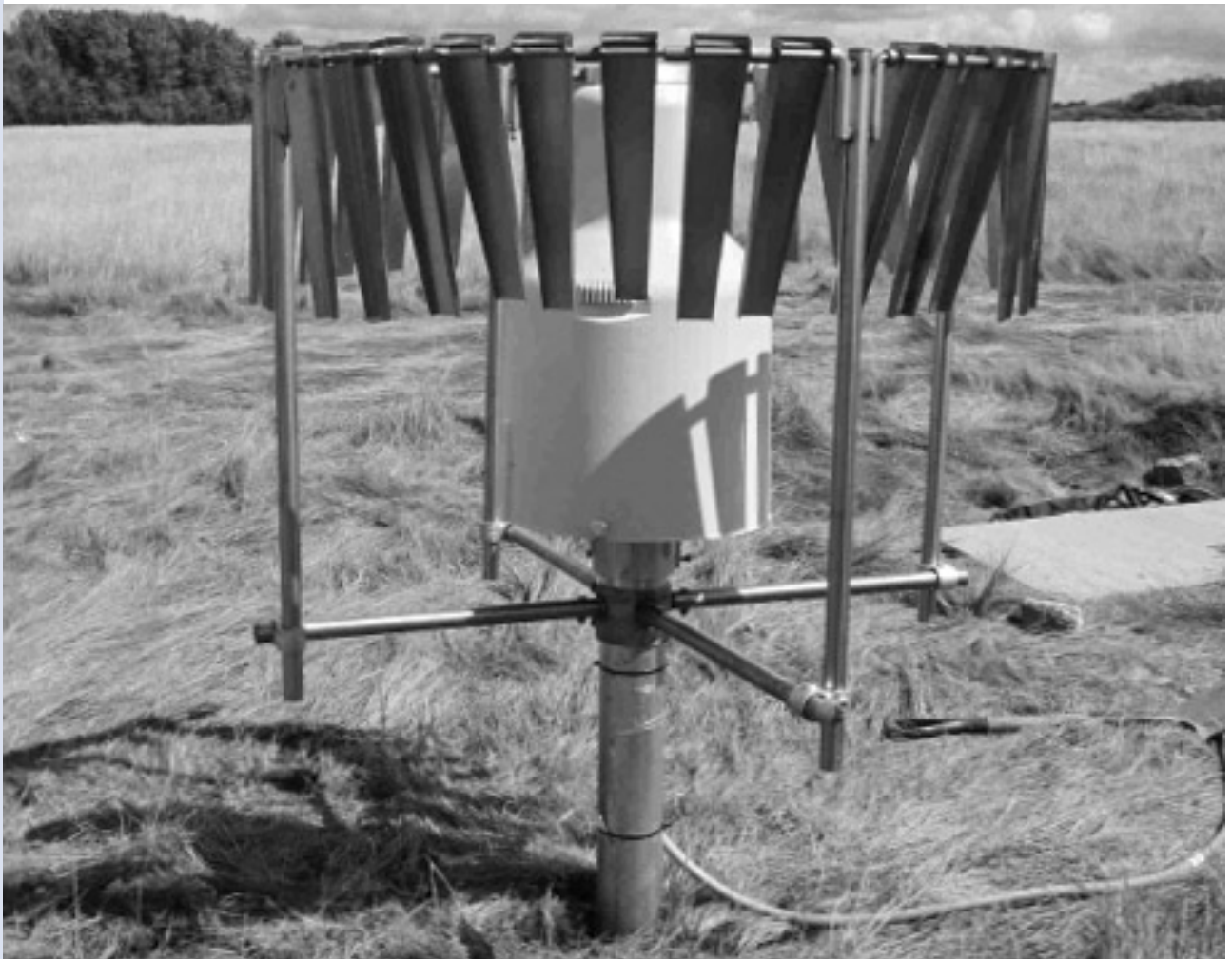
Figure 1: Rain gauge with wind screen
