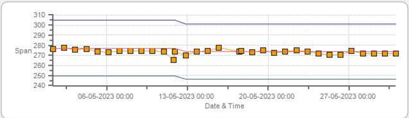
NO2[ppb] Calibration: Tamarack Monthly: 05-2023 Type: SpanAndZero - Span
