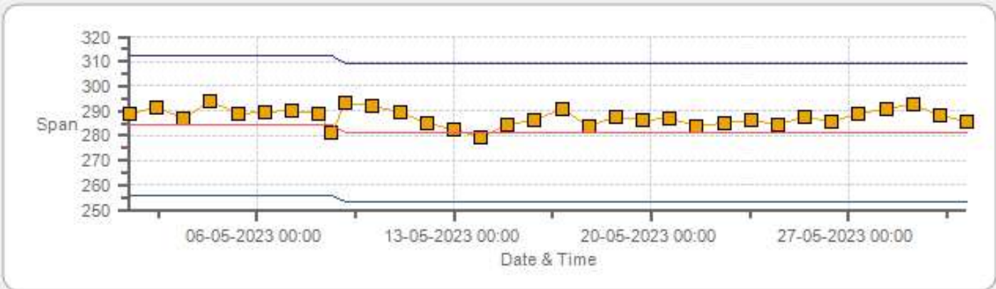
NO2[ppb] Calibration: Cold Lake South Monthly: 05-2023 Type: SpanAndZero - Span
