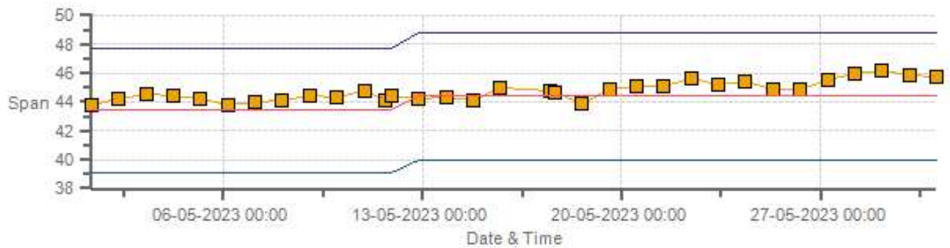
H2S[ppb] Calibration: Tamarack Monthly: 05-2023 Type: SpanAndZero - Span
