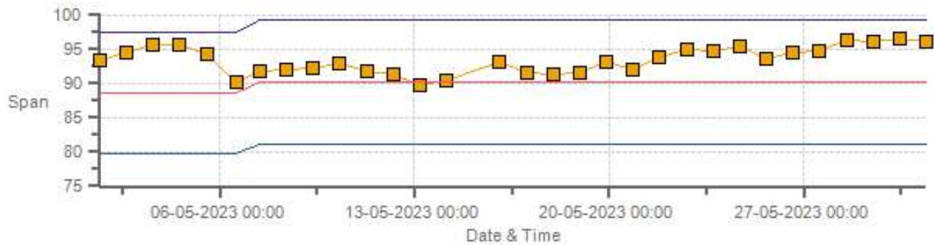
H2S[ppb] Calibration: St. Lina Monthly: 05-2023 Type: SpanAndZero - Span
