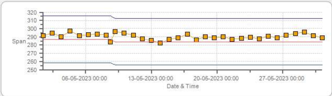
NOX[ppb] Calibration: Cold Lake South Monthly: 05-2023 Type: SpanAndZero - Span
