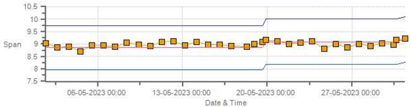
CH4[ppm] Calibration: Lac La Biche Monthly: 05-2023 Type: SpanAndZero - Span
