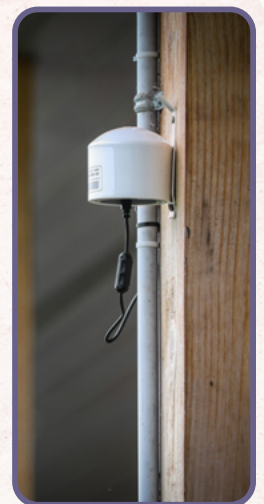
Small sensor for particulate matter monitoring
