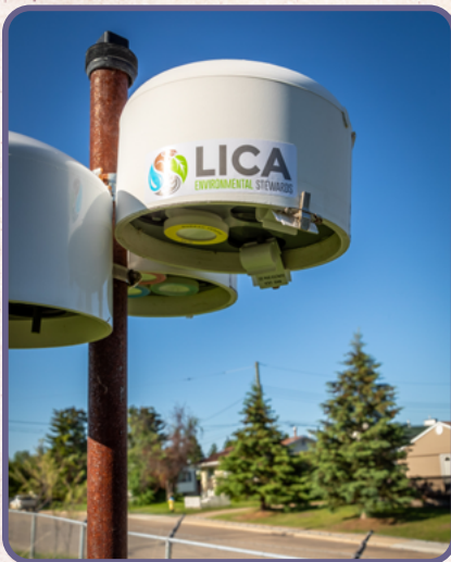
Station deployment showing sampling media in weather shelter
