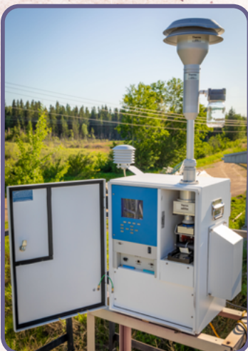
Partisol sampler - measures particulate matter concentrations
