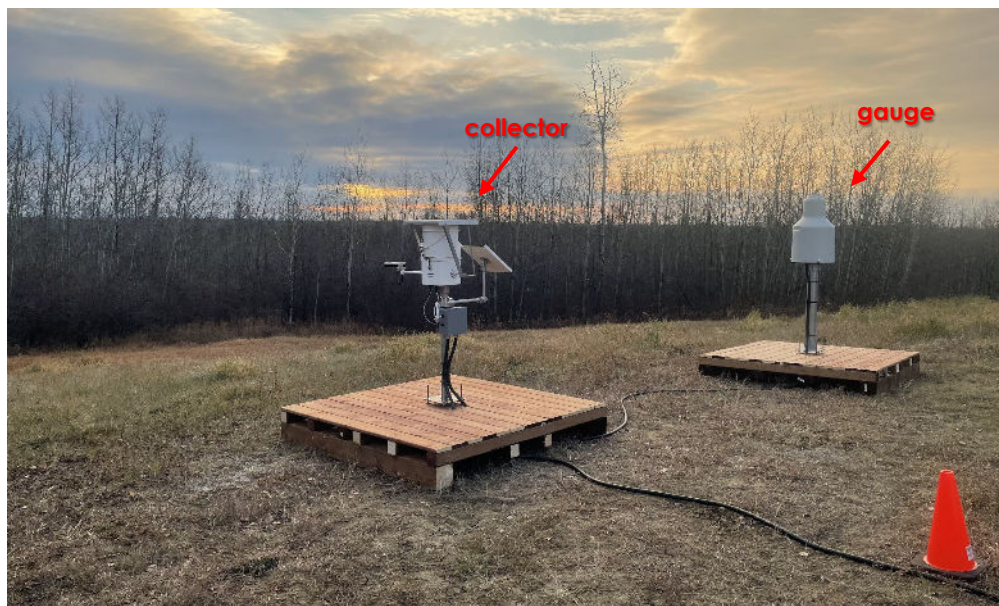
Figure 2: NCON precipitation collector (left) and Ott Pluvio precipitation gauge (right) deployed at St. Lina monitoring station.
